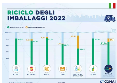
Figure 2.4 - Percentage of recycled packaging materials: steel, aluminium, paper, wood, plastic and bio-plastic, glass [ CONAI, 2022 ]
