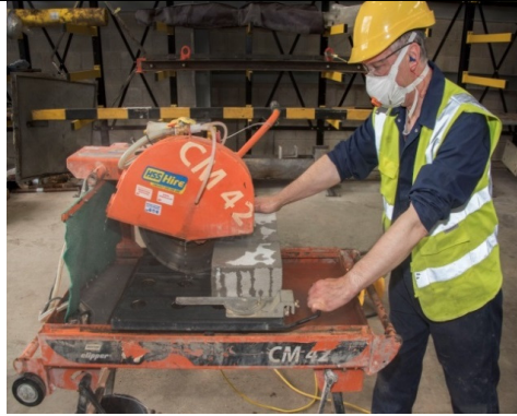
Good practice – Use of water suppression (shown) and RPE worn by the operator (HSE, GB)
