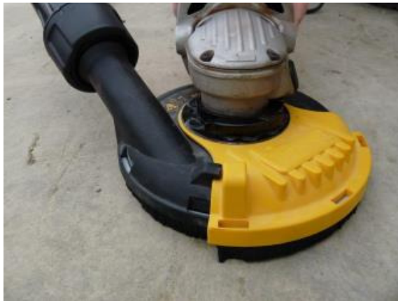
Figure 3 Grinder with on-tool extraction (Source HSE, GB)
